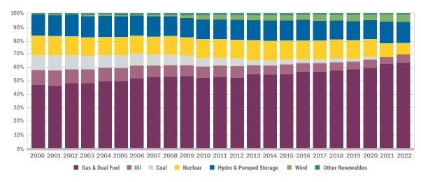
In New York State, we've seen these trends play out. The chart above shows that, since 2000, electric generators that primarily combust natural gas increased from less than 50% to more than 60% of the generating capacity in the state. That transition towards natural gas contributed to the complete phase-out of coal-fired generating capacity from the grid during this time frame.
