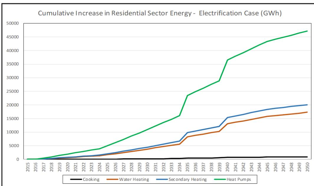
By far, the largest impact is conversion of fossil fuel heating systems to heat pumps and resistance heating backup or secondary heating. Figure 40 compares residential average use for the Reference, Policy, and CLCPA Scenarios.
