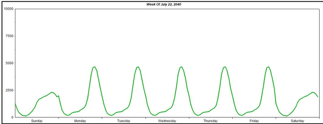
The Reference Case adjusted system load forecast is calculated by adding the electric vehicle hourly load forecast and subtracting out solar and battery hourly load forecasts. Figure 36 shows how adjustments for BTM solar and electric vehicles reshape system load over time.
