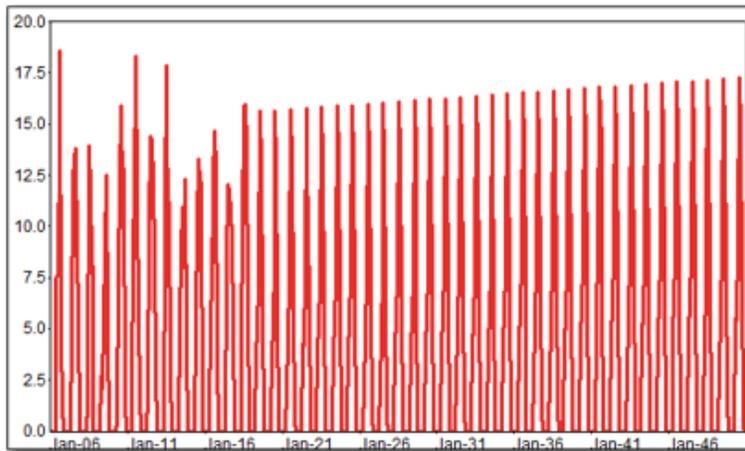
Trended CDD, HDD, and CTHI are used in constructing drivers for the forecast models. At the end of the process, the monthly CDD values increase during the forecast horizon and the monthly HDD values decrease during the forecast horizon, as shown in Figure 21 and Figure 22. The CDD values exhibit an increase of 0.8% annually (with a faster increase during the shoulder months than during the peak summer months), while the HDD values decrease by 0.5% annually.
