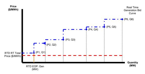
If the RTD interval LBMP (i.e., *RTD RT Total Price (\\$/MWh)*) is greater than the cost component of the last point on a Generator's Bid curve, depicted as  $P_6$  in the diagram below, then the Generator's EOP is equal to the megawatt component of the last point on the its cost curve (i.e.  $Q_6$ ).
