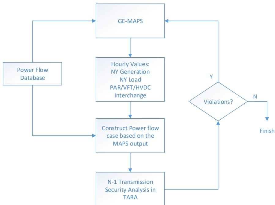
Figure 26 shows the flowchart for Roundtrip MAPS/TARA Analysis. This iterative analysis has three steps:
