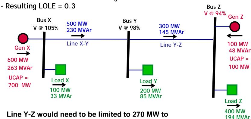
Line Y-Z would need to be limited to 270 MW to maintain 95% at Bus Z
