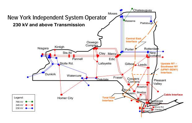
Transmission interfaces are groupings of transmission lines which measure the transfer capability between regions. The lines connecting Leeds and Pleasant Valley are known as the UPNY/SENY interface while the lines running south from Pleasant Valley and those from Ramapo to the cables feeding into New York City and Long Island are known as the UPNY/ConEd interface. These are the key transmission interfaces in the Hudson Valley.
