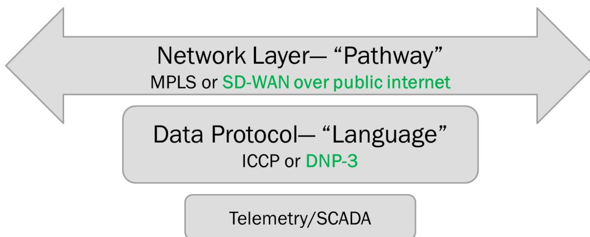
The current telemetry framework is a reliable solution, enabling the NYISO and Transmission Owners to have grid visibility, respond to disturbances, and efficiently meet demand at all times. The telemetry framework enables system operators to manage data and execute reliability functions as needed. Reliable telemetry encryption and communication supports current NYISO initiatives, and will continue to serve a key role in NYISO operations going forward.
