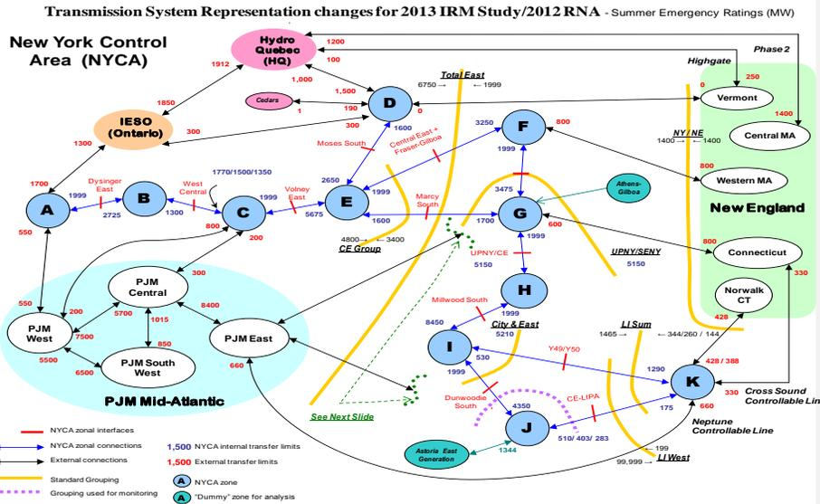
**Figure 4-2 Transmission System Representation for MARS modeling**
