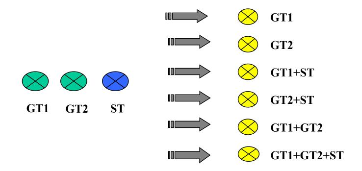
Proposed modeling approach represents the allowable potential plant configurations as "pseudo units" and additionally represents transitional limits and costs between the allowable plant configurations
