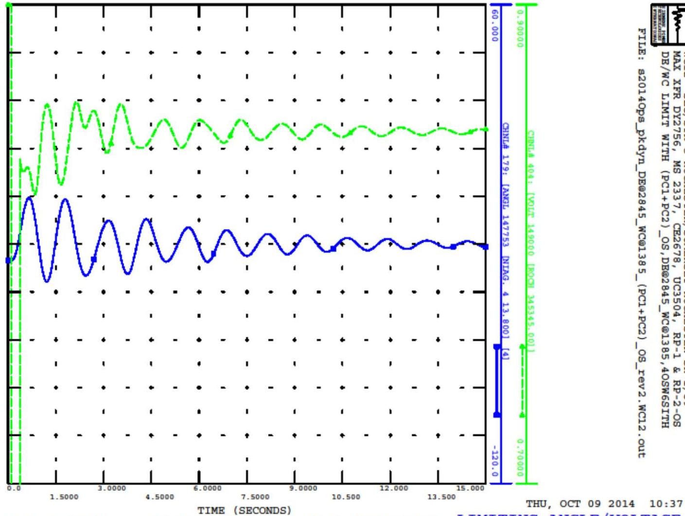
Fig 12 Angle/Voltage response for Pannel - Clay (PC1) & Pannel - Clay (PC2) 345 kV O/S
