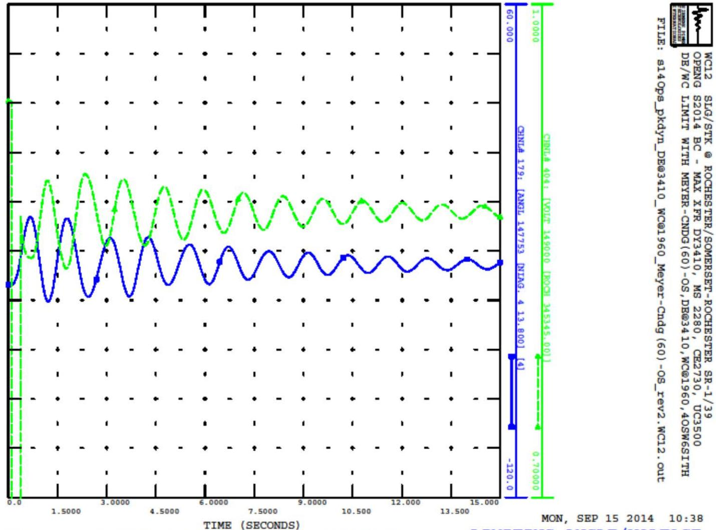
Fig 3 Angle/Voltage response for Meyer - Canadiqua (60) 230 kV O/S
