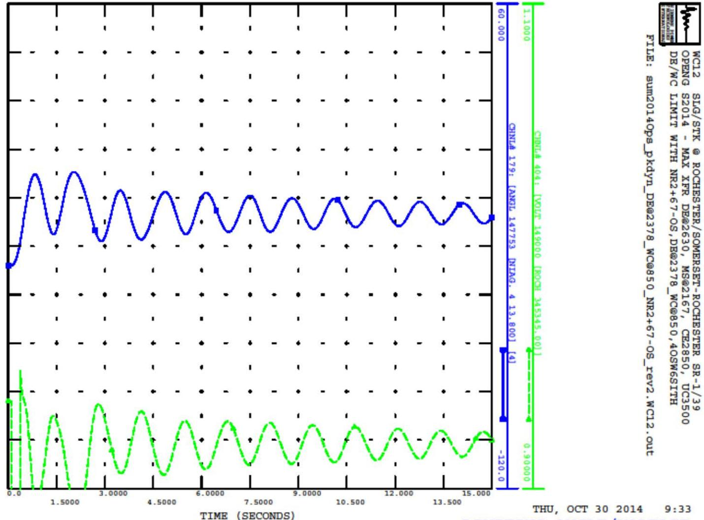
Fig 9 Angle/Voltage response for Niag- Roch (NR2)& Stole Rd-Shldn (67) 345 kV O/S
