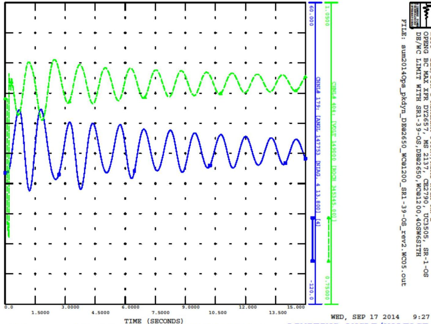
Fig 5 Angle/Voltage response for Sommerset- Roch (SR1-39) 345 kV O/S
