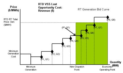
$LOC_{Cost}^{RT}$ : Costs avoided by Generator g from being instructed to reduce its Energy output to provide Voltage Support Service, determined as illustrated below:
