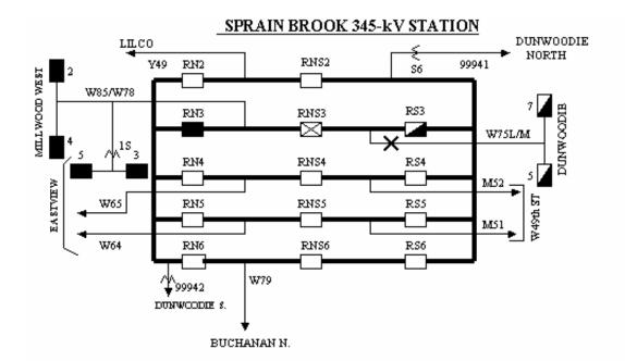
DESCRIPTION: SINGLE-LINE-TO-GROUND FAULT WITH DELAYED CLEARING AT SPRAIN BROOK 345-kV STATION ON FEEDER W75L/M
