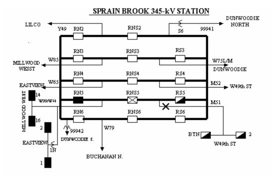
DESCRIPTION: SINGLE-LINE-TO-GROUND FAULT WITH DELAYED CLEARING AT SPRAIN BROOK 345-kV STATION ON FEEDER M51
