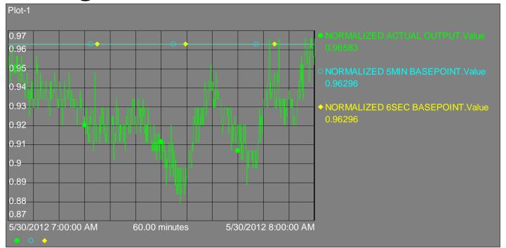
Above: Historical generation output from a refuse burning generator in NYCA, with 5 min and 6 sec base points from the ISO. All values are normalized by the maximum operating limit.
