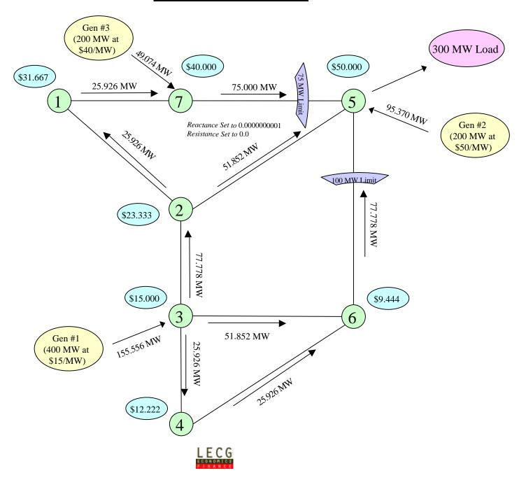
The third scenario is identical to Scenario 1 but schedules on the controllable line are determined by the ISO. The illustration again assumes that generation is available for dispatch at Buses 3, 5 and 7.
