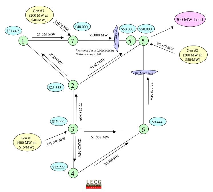
It can be seen that construction of the controllable line increases transfer for capability by more than the 75 MW scheduled to flow on the controllable line.
