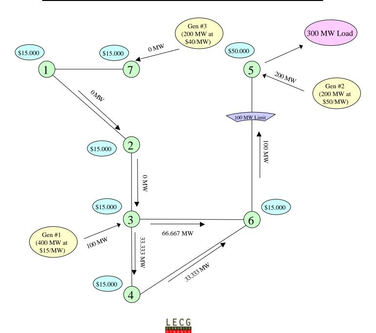
Absent the controllable line, transfer capability from Bus 3 to Bus 5 would be 100 MW, limited by the flows on line 6-5 in the contingency in which line 2-5 is out.
