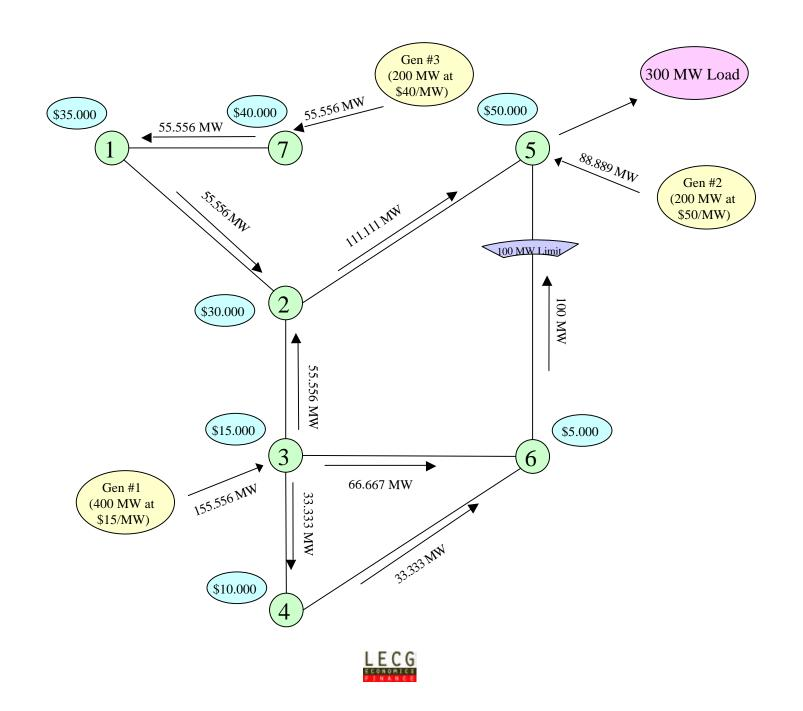
In Scenario 2, however, the outage of the controllable line is also a binding contingency. As a result, the proxy price for deliveries over the controllable line would be less than the value of generation at Bus 5, because of the impact of schedules over the controllable line on the constraint in the contingency in which the controllable line is out.
