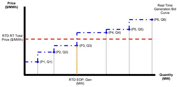
If the RTD interval LBMP intersects the given Generation Bid block on a horizontal line and the Generator's RTD Base Point is greater than the megawatt component of the last point on the Generator's bid curve, as in the diagram below, then the Generator's EOP is equal the its RTD Base Point.
