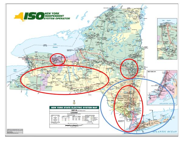
Note: The red circles indicate the areas where the load may be impacted by transmission security constraints, and the blue circle indicates the region with resource adequacy violations.
