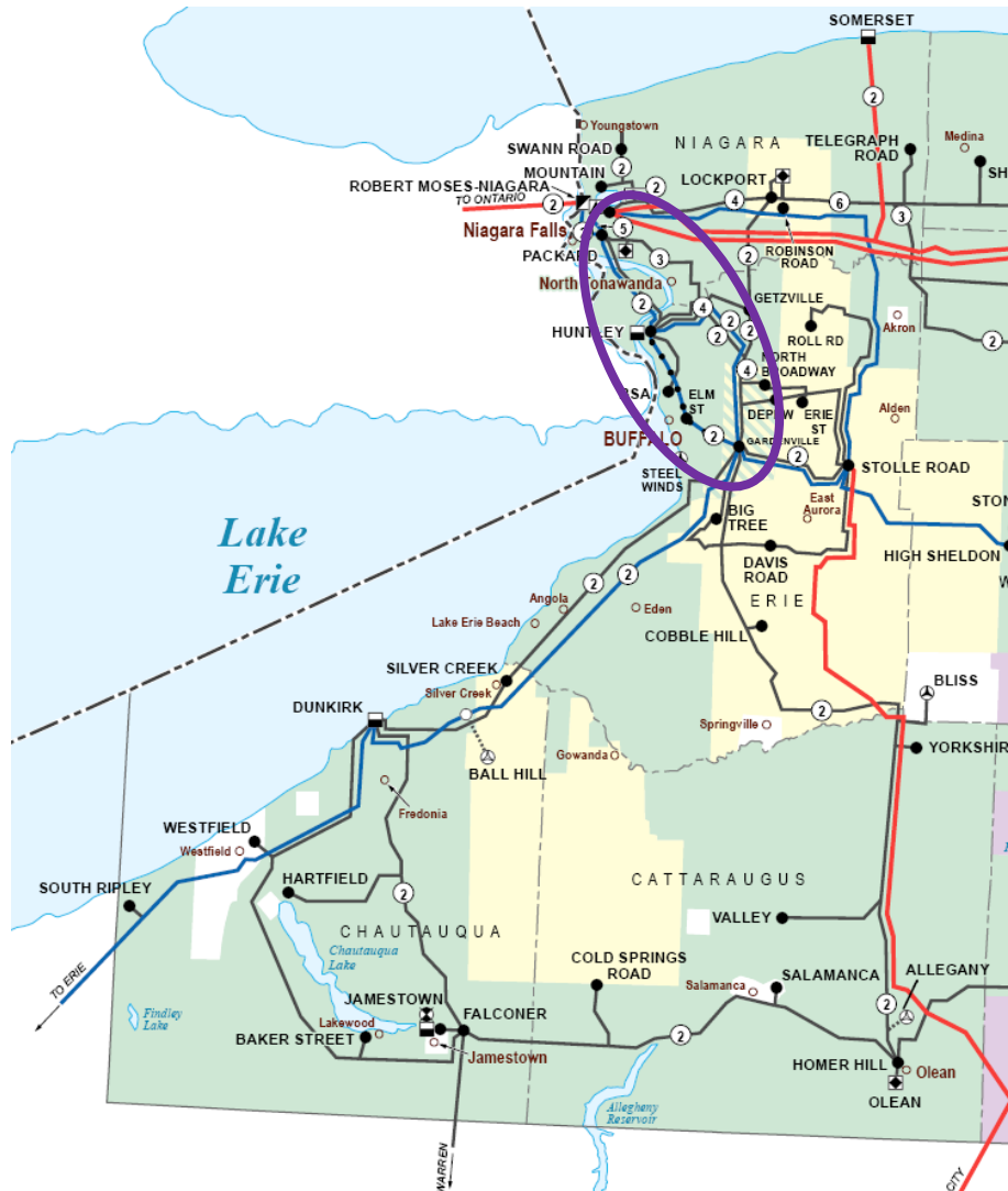
Key: red lines = 345kV; blue lines = 230kV; black lines = 115kV Purple circle = constrained 230 kV lines
