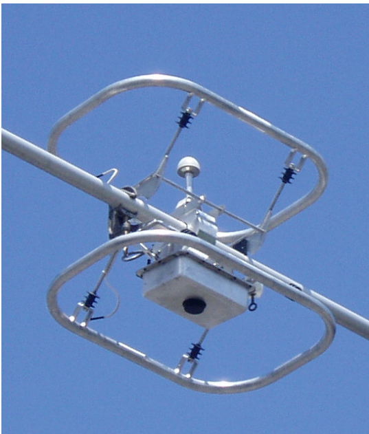
Figure2. Self-power HV Primary Sensor (left) and Figure 3, the Battery Powered Primary Sensor (above)
