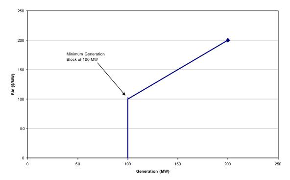
The unit has a minimum generation block of 100 MW and an incremental energy curve with a slope of 1 from 100 MW to 200 MW. The unit has a ramp rate of 1 MW/minute.
