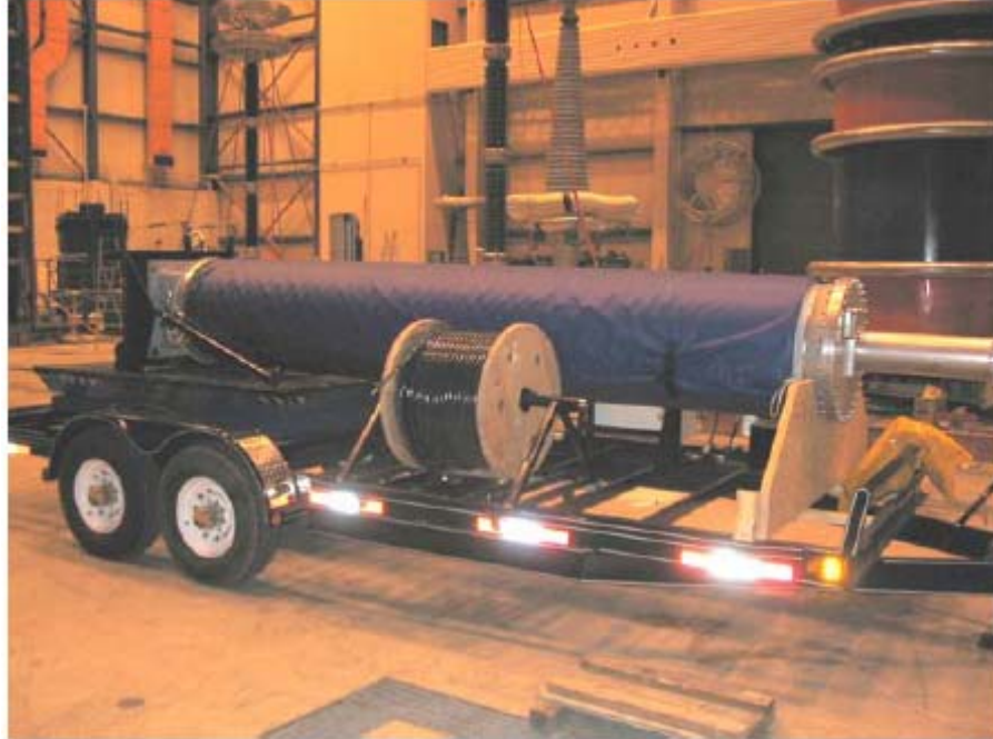
Figure 1: Portable OVT reference using a 500 kV optical VT
