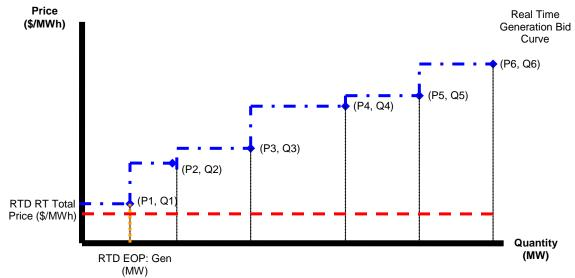
If the RTD interval LBMP (i.e., *RTD RT Total Price* (\$/MWh)) is greater than the cost component of the last point on a Generator's Bid curve, depicted as  $P_6$  in the diagram below, then the Generator's EOP is equal to the megawatt component of the last point on the its cost curve (i.e.  $Q_6$ ).
