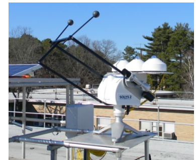
Sun tracker with sensors for global, diffuse and direct Irradiance.
