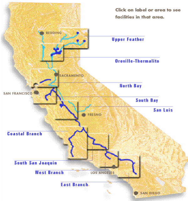
Figure 8 The geographic diversity of the CDWR pumping system makes it a valuable spinning reserve resource capable of responding even if there are congestion constraints.
