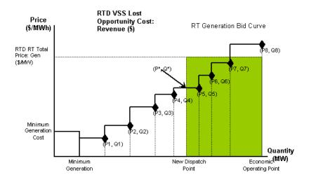
$LOC_{Cost}^{RT}$ : Costs avoided by Generator g from being instructed to reduce its Energy output to provide Voltage Support Service, determined as illustrated below:
