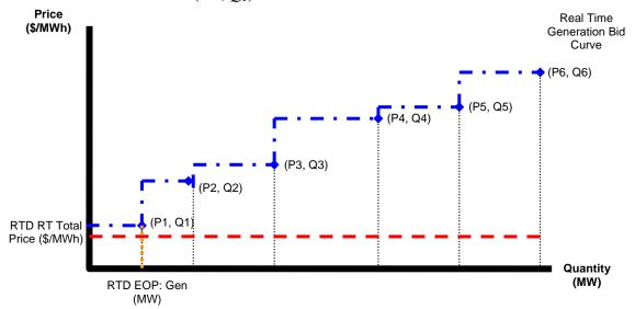
If the RTD interval LBMP (i.e., RTD RT Total Price (\$/MWh)) is greater than the cost component of the last point on a Generator's Bid curve, depicted as  $P_6$  in the diagram below, then the Generator's EOP is equal to the megawatt component of the last point on the its cost curve (i.e.  $Q_6$ ).
