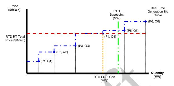
In the diagram below, the RTD interval LBMP intersects the given Generation Bid block on a horizontal line and the Generator was Base Pointed below the given Generation Bid block. In this case, the Generator's EOP is equal to the lower Generation Block MW (i.e.,  $Q_3$ ) of the block where the RTD interval LBMP intersects the Generation Bid.
