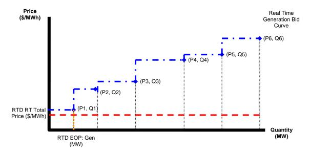
If the RTD interval LBMP (i.e., RTD RT Total Price (\$/MWh)) is greater than the cost component of the last point on a Generator's Bid curve, depicted as  $P_6$  in the diagram below, then the Generator's EOP is equal to the MW component of the last point on the its cost curve (i,e,.  $Q_6$ ).
