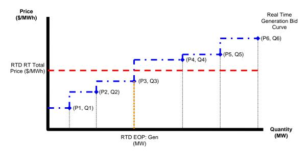
If the RTD interval LBMP intersects the given Generation Bid block on a horizontal line and the Generator's RTD Base Point is greater than the MW component of the last point on the Generator's bid curve, as in the diagram below, then the Generator's EOP is equal the its RTD Base Point.
