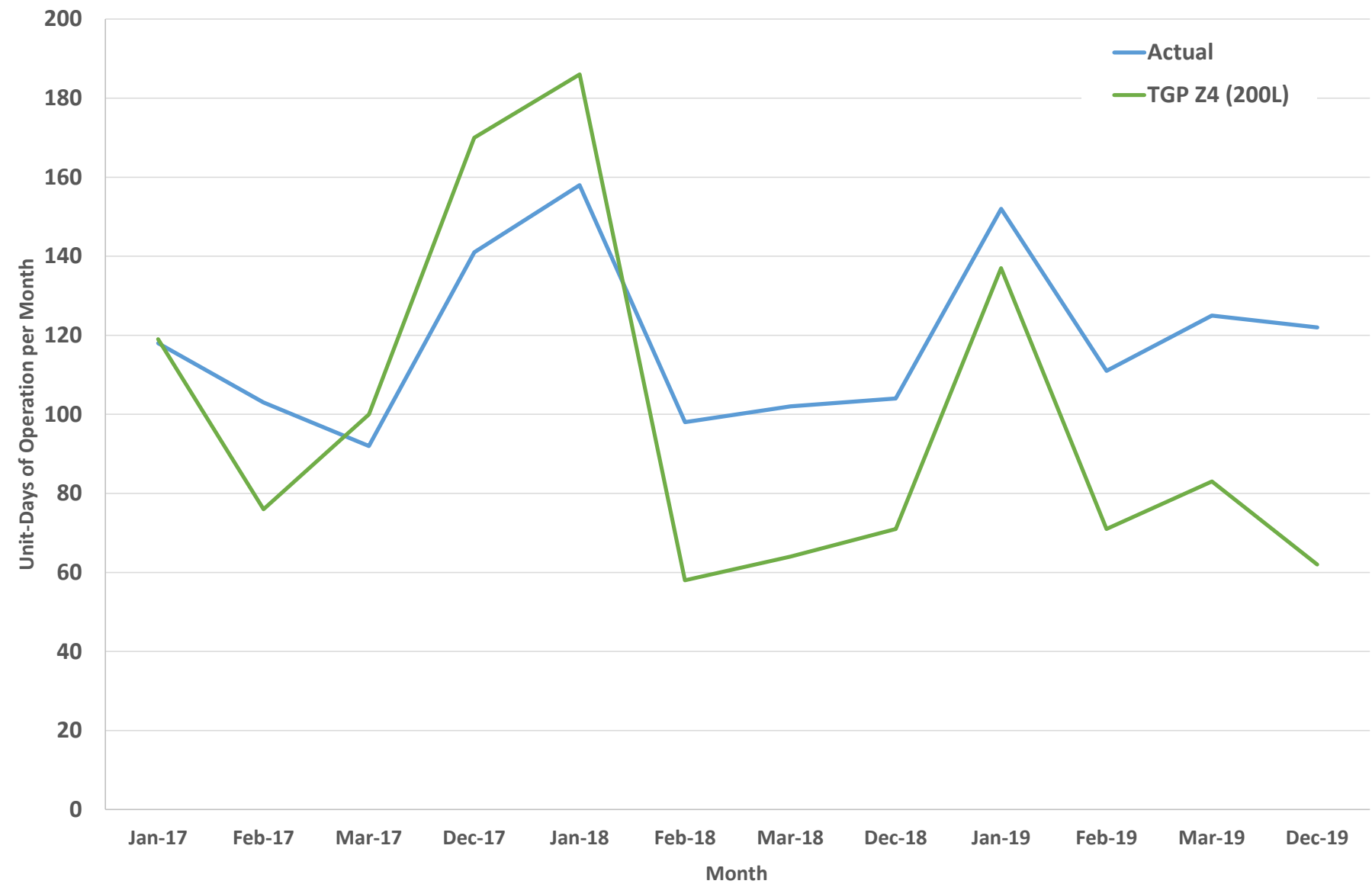
Fig. 3: Historical vs. Backcast Operation for Zone C Gas-Fired Plants in Dec. through March, Using TGP Zone 4 (200L) Price Index for Backcast Simulation
