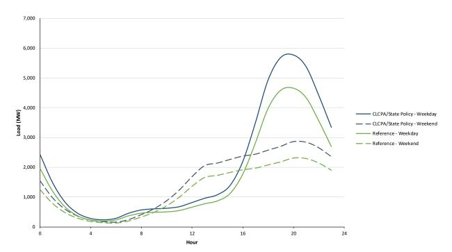
Figure 7: Electric Vehicle Daily Load Shape from Phase I Study
