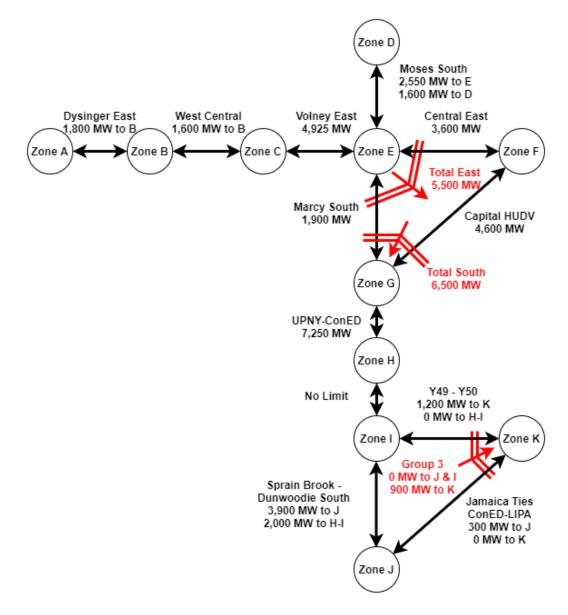
Figure 9: Simplified Transmission Map and Limits, Starting Point
