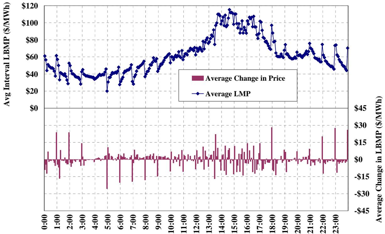
This figure shows that most real-time price fluctuations occurred predictably at specific times of the day, particularly near the top of the hour during ramp-up and ramp-down hours. In the last
