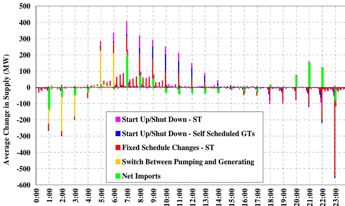
The figure shows adjustments in net imports, pumped storage units switching between pumping and generating, and adjustments in fixed generation schedules accounted for the most significant changes in inflexible supply from interval-to-interval in 2010. For example, from 10:55 pm to 11:00 pm, the average net decrease in inflexible supply from imports and fixed scheduled units was more than 545 MW, coinciding with a \$28/MWh average increase in real-time clearing prices.
