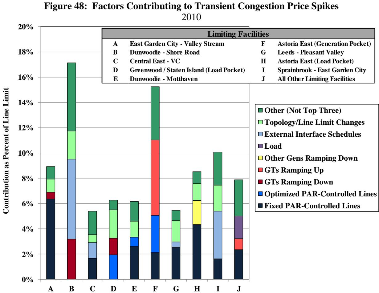
The figure shows that Fixed PAR-Controlled Line flow changes were the most significant factor contributing to transient shadow price spikes in 2010. This was the top contributing factor for six of the ten facility categories shown in the figure, including:
