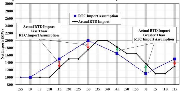
Figure A-72: Illustration of External Transaction Ramp Profiles in RTC and RTD
