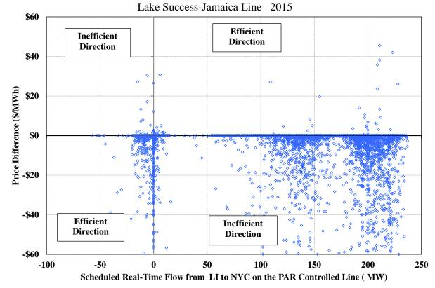
Figure A-78: Efficiency of Scheduling on PAR Controlled Lines
