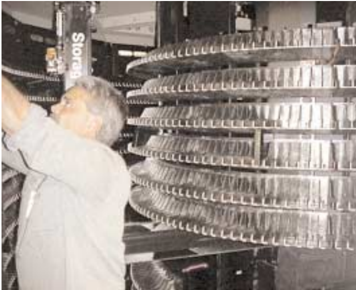
A technician works on a Storage Tek tape silo, capable of holding 2,000 computer storage tapes containing 240,000 gigabytes or more than three years of market information. During 2000, the NYISO greatly upgraded its information technology systems, increasing the number of servers and work stations from 100 to 155.
