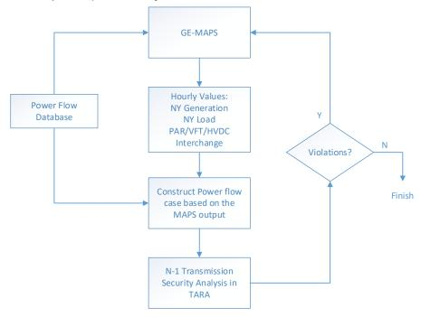
Figure 60 shows the flowchart for Roundtrip MAPS/TARA Analysis. This iterative analysis has three steps:
