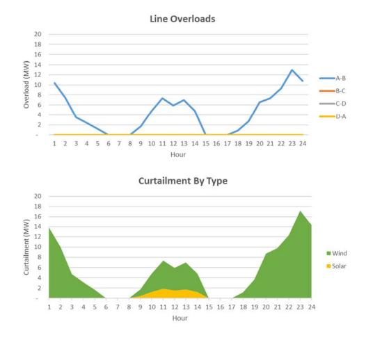
Note that, for this example system, if only one of the technology types is producing energy at the time of line overloads, the amount of curtailment necessary to remedy line overloads will exceed the overload amount. This is due to a particular generators shift factor relationship to the overloaded line. The interrelationship between the specific unit or units operating in a given period and the required level of curtailment to bring the system within criteria will be captured.
