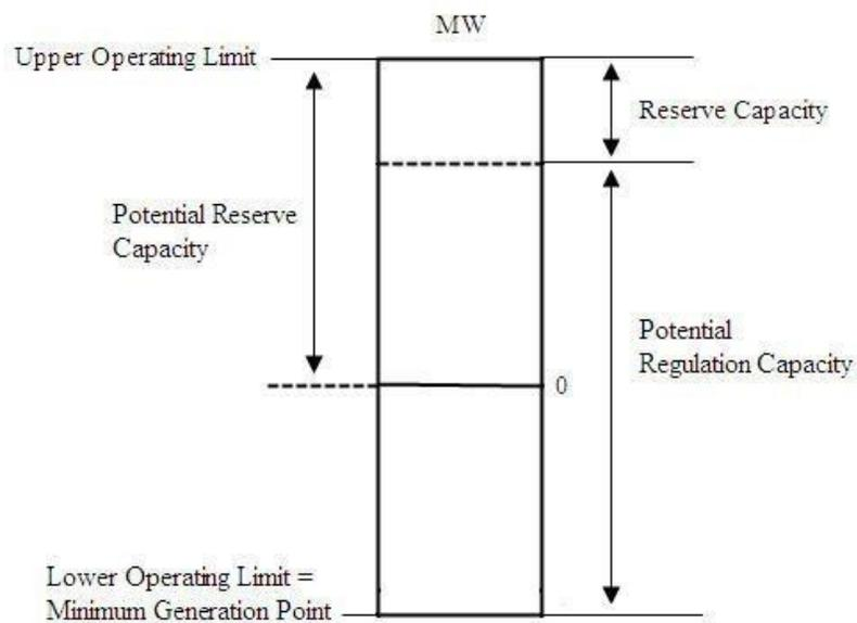
**Figure 6: Generating Unit Operating Characteristics**
