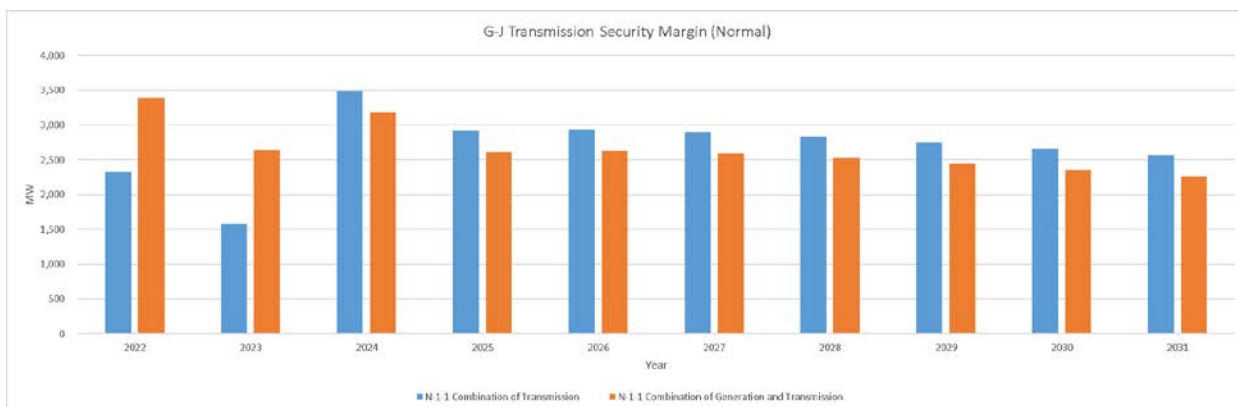
Figure XX:11: Lower Hudson Valley Summer Transmission Security Margin (Summer Baseline Peak Forecast - Normal)
