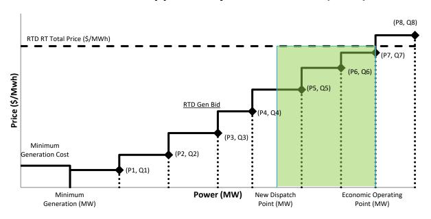
$LOC_{gi}^{RT}$ : Costs avoided by Generator g from being instructed to reduce its Energy output to provide Voltage Support Service, calculated as follows:
