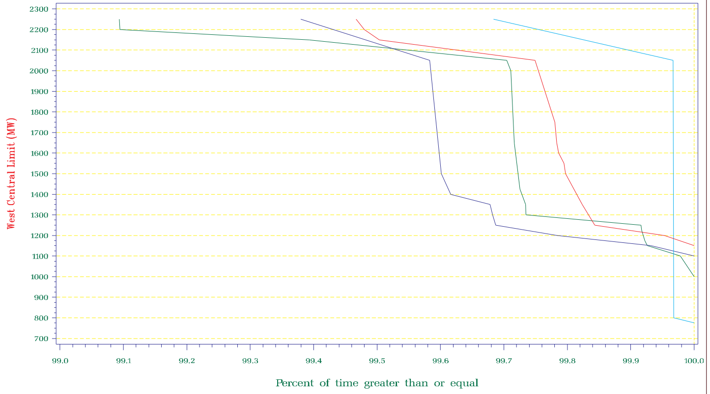
NYISO Percent of time Interface Flow For January 1998 – December 2001 West Central Limit
