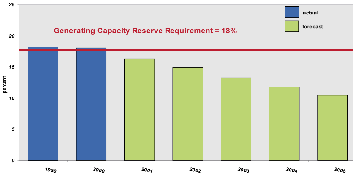
The above chart shows the State's looming generation shortage as projected in 2001
