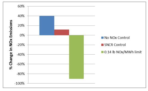
Figure 4-36: Example of CHP Displacing Central Generation in NY State: NO<sub>x</sub> Emissions
