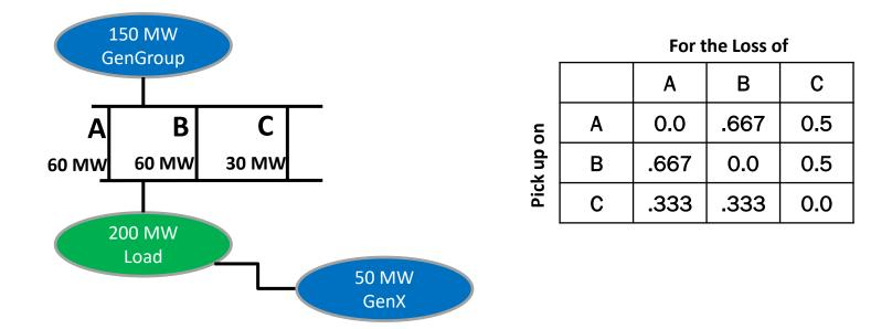
Secure for the loss of A, B or C. GenX is constrained "on" for security.
