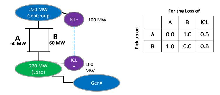
A and B cannot pick up the load securely for the loss of any single element.
