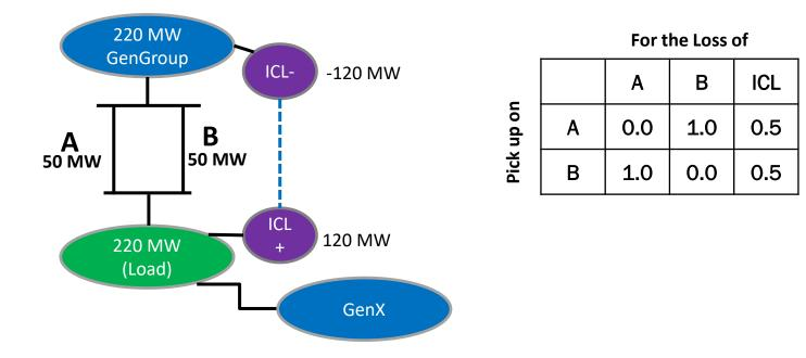
ICL cannot pick up the load as A and B not secure for the loss of ICL
