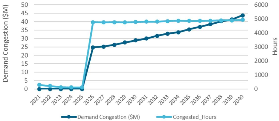
This line is congested very little prior to 2026 but the congestion increases significantly after offshore wind project is modeled in-service. The unit is injecting at a lower kV bus which is not designed to handle the amount of power produced by a large project. The violin plots below show a significant increase in line utilization starting in 2026 across all seasons.
