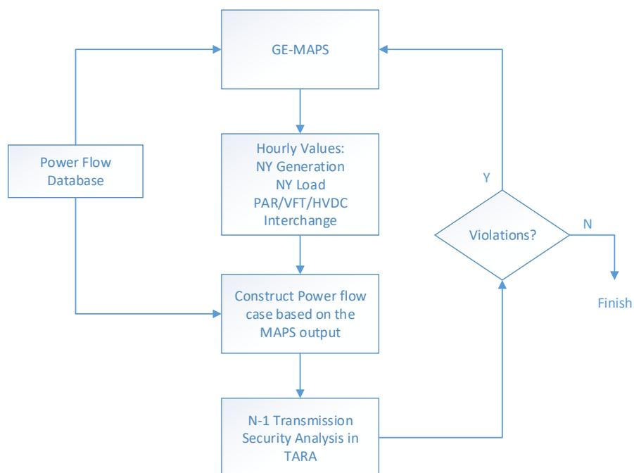
Figure 25 shows the flowchart for Roundtrip MAPS/TARA Analysis. This iterative analysis has three steps:
