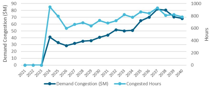
Line utilization on Sugarloaf-Ramapo 138 kV increases slightly during the summer period compared to the Baseline Case line utilization. The flow utilization in this path significantly increased with a portion of Segment B of the AC Transmission Public Policy project in-service in 2024. Higher flow utilization is observed in summer and fall because the seasonal rating is lower than in winter period.
