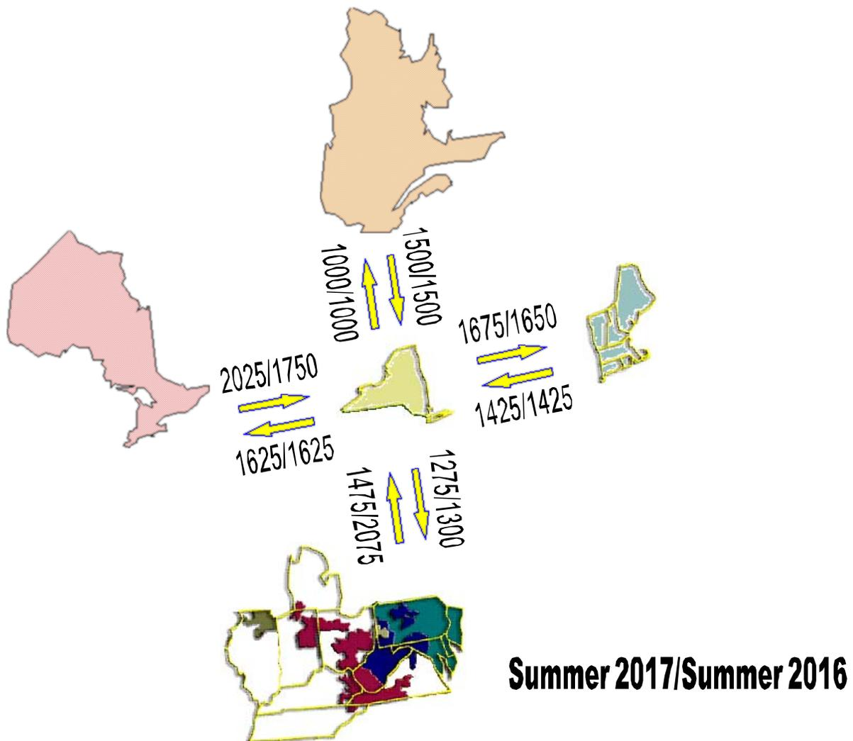
**Figure 2 - Inter-Area Thermal Transfer Capabilities<sup>3</sup>**
