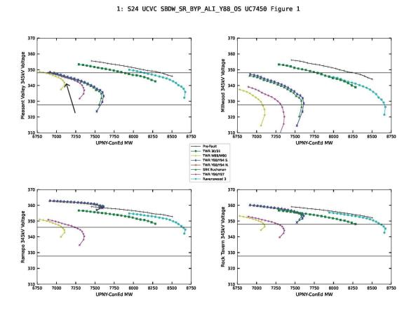
Figure 10 below shows the pre-contingency base flow with respect to the post contingency voltage for each of the most limiting contingencies. The graph is marked with at the MW level corresponding to the knee of the curve from the previous post-contingency plot. It is also marked at the MW level of the 5%
