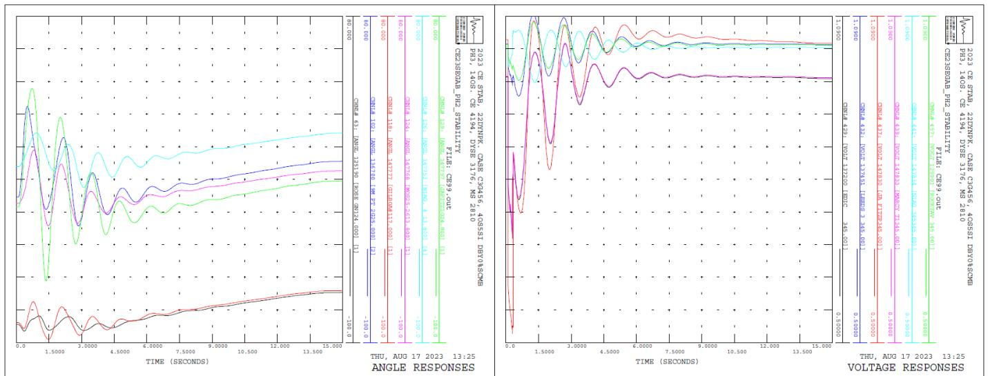
Figure 10: 14 Line Out-of-Service Angle and Voltage Response to CE99
