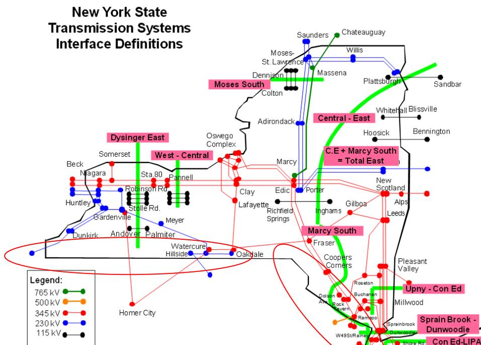
Figure 1. NYCA Transmission System Interface
