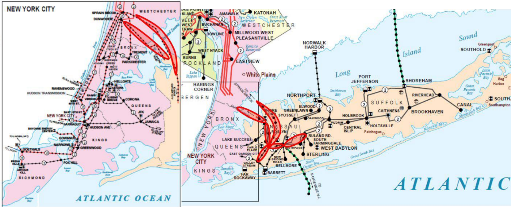
Figure 1: Significant N-0 Constraints. Red shading indicates constraints that occur in the light load conditions.
