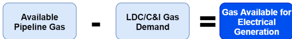
Figure 8: Diagram of Natural Gas Model
