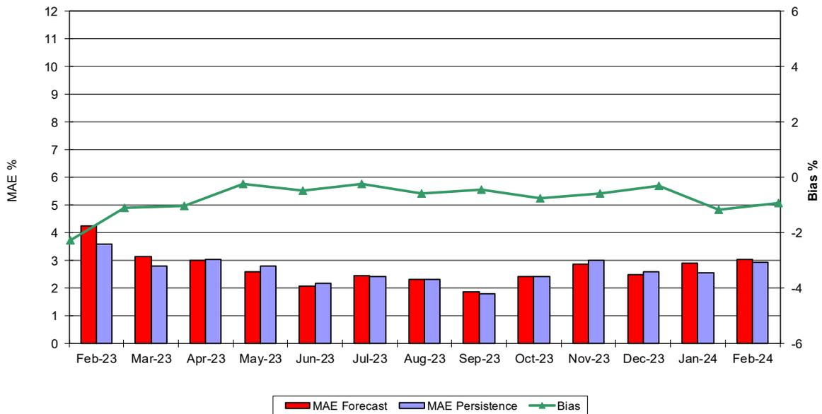
**MAE Forecast** - Avg |actual wind generation - hour ahead forecast wind generation| / Wind Capacity
