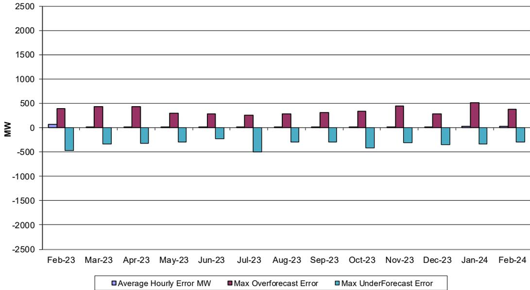
**Hourly Error MW** - Value of the difference between the hourly average actual wind generation and the average hour ahead forecast wind generation.
