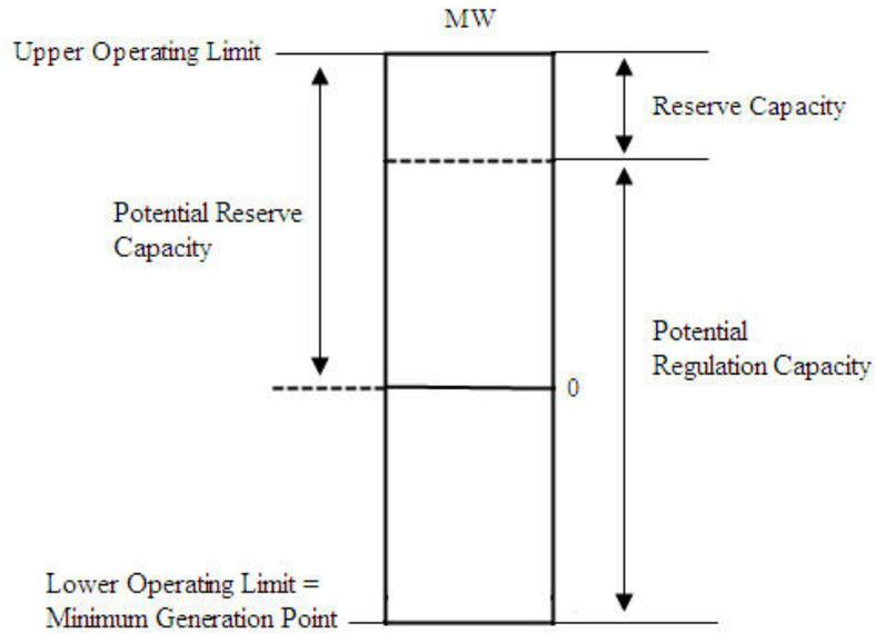
**Figure 6: Generating Unit Operating Characteristics**
