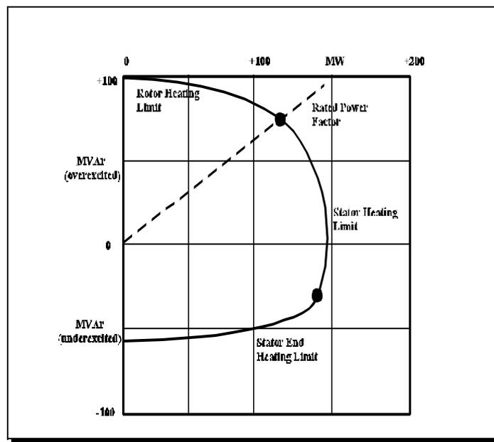
The ability of a generator to produce or absorb Reactive Power (MVA<sub>r</sub>) is limited by generator heating considerations. At full load, a generator is able to produce or absorb a relatively small amount of Reactive Power. As the generator’s production of real power decreases, its ability to produce or absorb Reactive Power increases. Figure 3, called a reactive capability curve or a D-Curve, is representative of generators limiting characteristics at a particular temperature. Reactive
