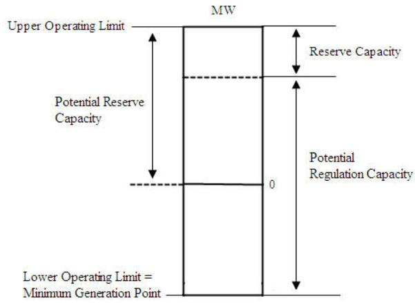
**Figure 6: Generating Unit Operating Characteristics**
